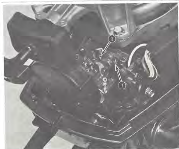
Fig How the motor can be made to idle without use of the throttle
